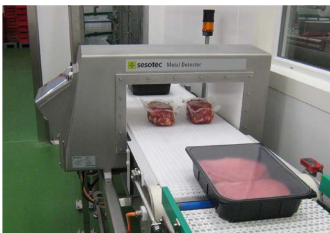
The metal detector INTUITY with multi-simultaneous-frequency technology in the inspection of very different products.
